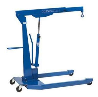
•A Hydraulic Floor/Engine Crane (also referred to as an engine hoist) is a common repair tool used in vehicle repair shops to remove or install gasoline or diesel engines in small and crowded vehicle engine compartments.
